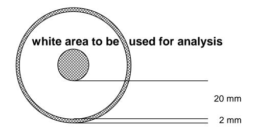
Primary intended use for STP Reference Materials is the optical emission spectrometry. Other applications are X-ray fluorescence spectrometry (XRF) and classical wet chemical procedures. Calibration measurements should be limited to the white area as defined on the above sketch.
